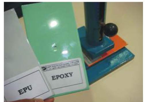
Impact test is being done on epoxy & epu panels. Epoxy coating breaks, while epu is resilient
